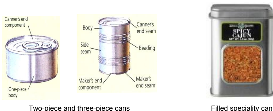
Figure 15. Two-piece and three-piece cans and speciality steel cans
